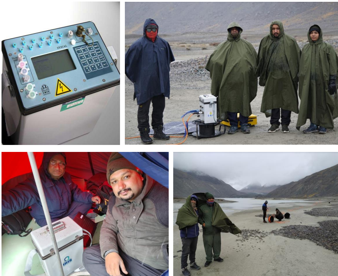
A glimpse of field observations via Syscal Pro resistivity measurement at Samundra Tapu Glacier (Lahaul & Spiti, HP).
