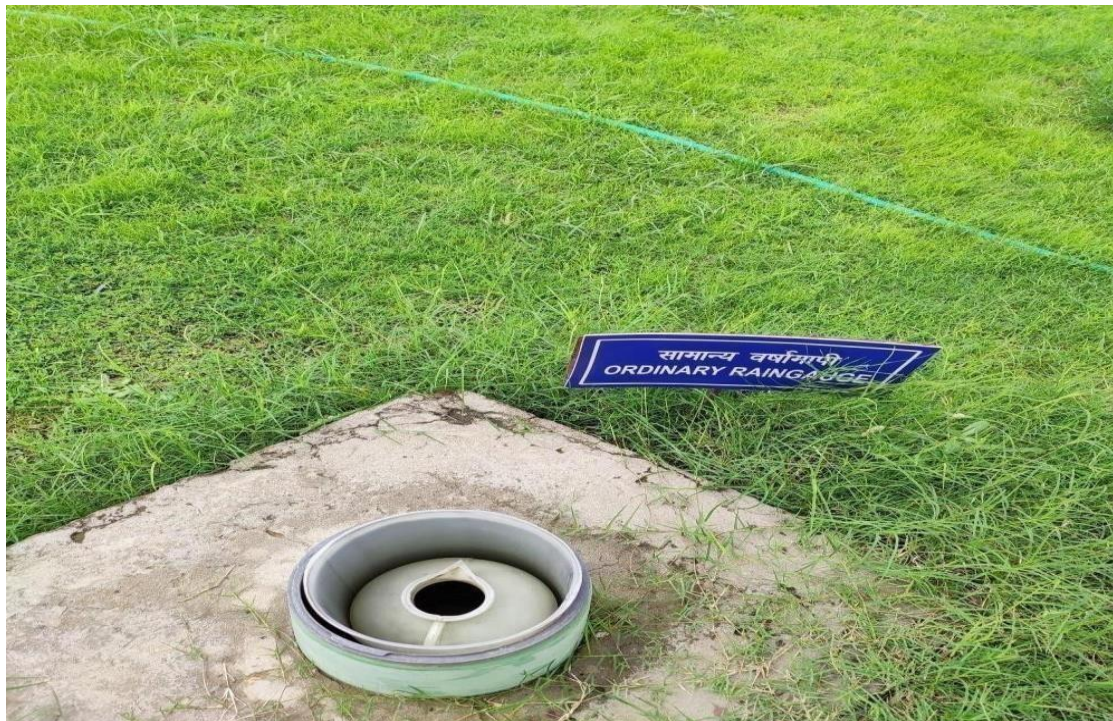
Fig. 5.7: Ordinary Rain Gauge
