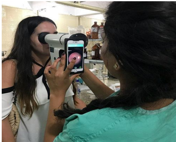
Figure 2: Fundus Camera integrated with Smart Phone [24]
